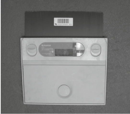
Figure 13.11 Computed radiography detector plate. The image plate has been partially removed from the protective cover.
